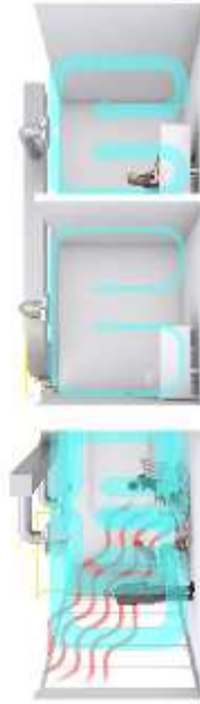
A diffuser can provide personalized airflow zones.
